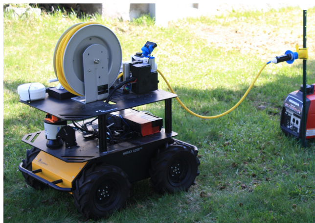
Fig. 1. An Autonomous Mobile Microgrid UGV deploys a power cable to connect a genset power source to an infrastructure load.
