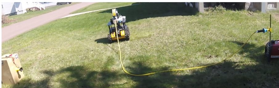
Fig. 12. A demonstration video of the ACMM on a UGV includes, from left to right, an infrastructure load, the cable following the track of the UGV through the environment, and a genset.
